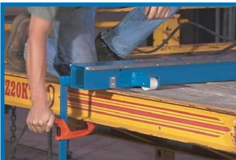
Quick action clamps make set-up fast and flexible!
