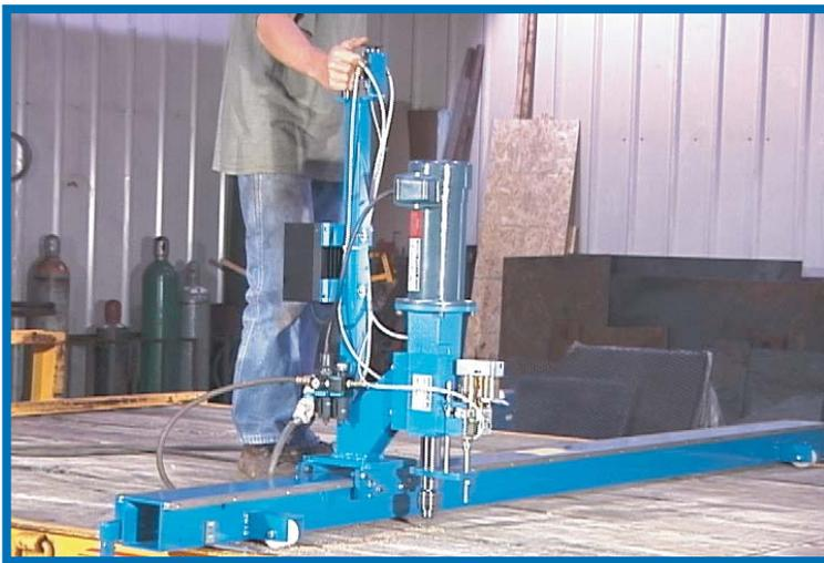
The Drill Unit glides across the width of the deck on ball bearing rollers. One push of the button advances the drill through the wood and the steel cross member, then it automatically retracts.
